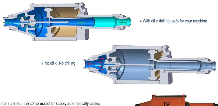
It oil runs out, the compressed air supply automatically closes Reliable operation is guarranted Safety off function if air disconnects
